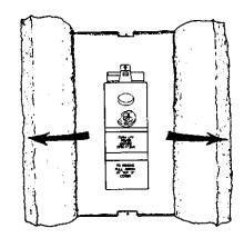
6. Lift out the tab as shown to unclip the terminal cover from the thermostat. The terminal cover can now be removed from the thermostat.
